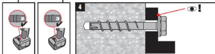
Installation with other electrical impact screw drivers of equivalent force and performance is possible.
