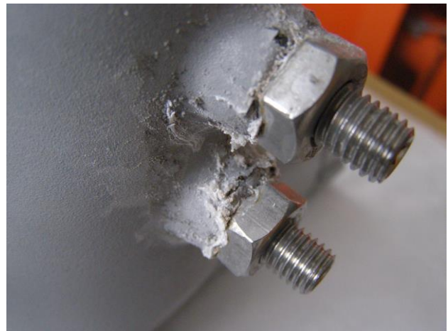
# Picture 4: Holder lamps with mounting screws after 1000 hours of NSS
