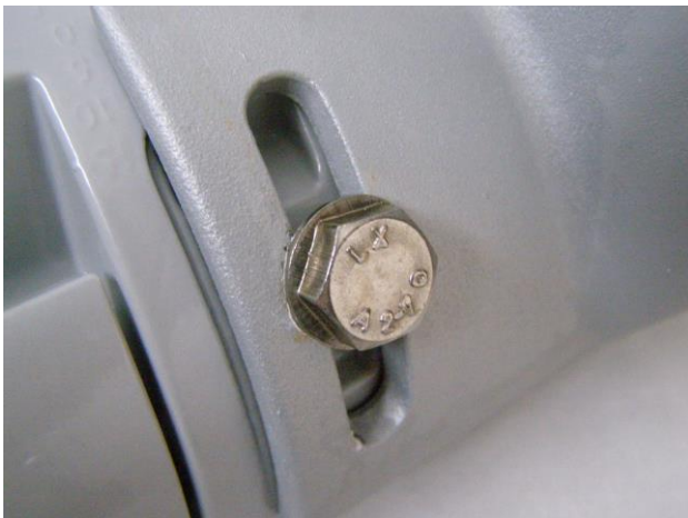
# Picture 3: Screw after 1000 hours of NSS
