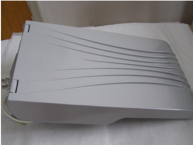
# Picture 1: LED street lamp Luxtella - upper side, after 1000 hours of NSS
