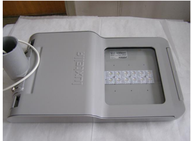
# Picture 2: LED street lamp Luxtella - lower side, after 1000 hours of NSS
