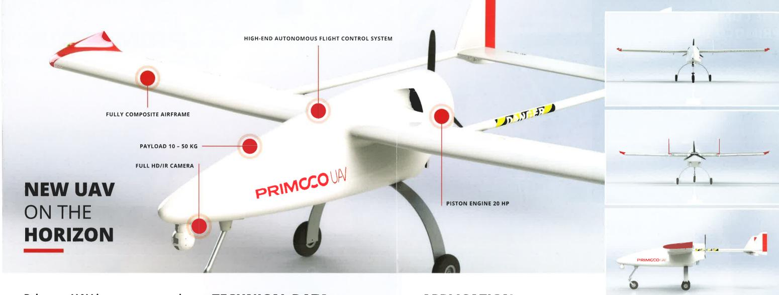
Primoco UAV is an unmanned aircraft which can be handled remotely or fly independently based on the programmed flight plans. With its very short distance take-off and landing, it ranks with the category STOL (Short Take-off and Landing).
