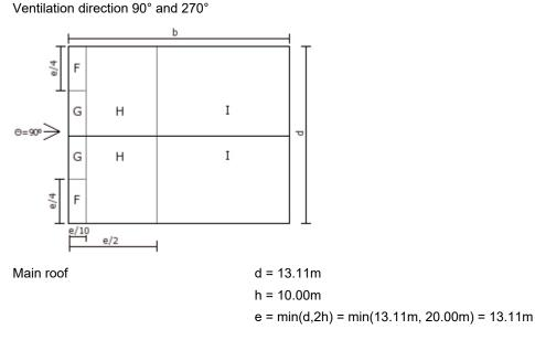
The coefficients for pressure and suction for the corresponding roof areas and a roof pitch of 35° are interpolated from the tables of EVS-EN 1991-1-4/NA:2007 for Pitched and butterfly roofs. With this, 1,95 m<sup>2</sup> is set as a value for the load introduction surface.
