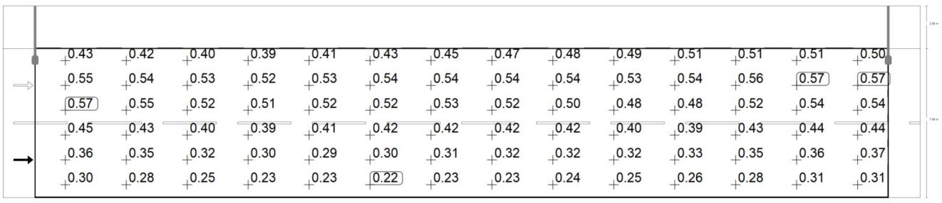
Observer 1: Luminance with new installation [cd/m 2 ] (Value grid)
