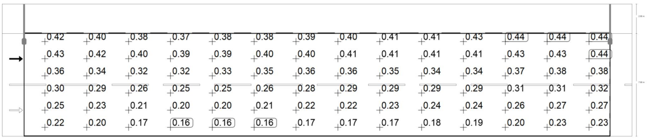
Observer 2: Maintenance value, luminance with dry roadway [cd/m 2 ] (Value grid)
