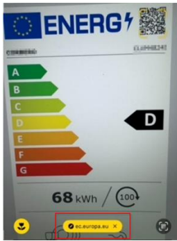
Figure 2: The QR code as feature on all modernised/newly introduced labels under the ELR. Scanning it leads to the full information registered in EPREL
