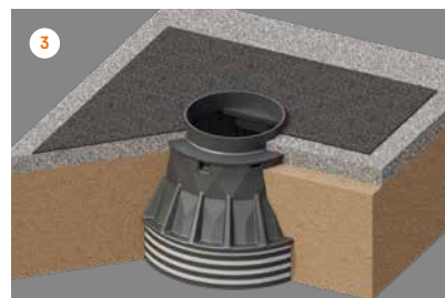
3 Paigaldada tasanduskiht.
